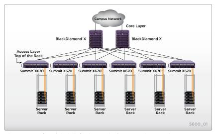
Figure 1: Top of Rack Switch for Servers in the Enterprise Data Center
