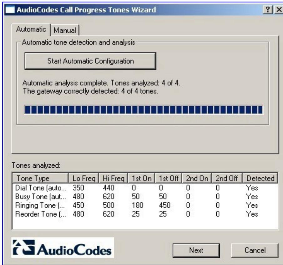
6. All four Call Progress Tones are saved (as standard A-law PCM at 8000 bits per sample) in the same directory as the CPTWizard.exe file is located, with the following names:
