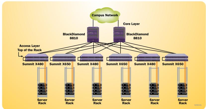
Figure 10: Top-of-Rack Architecture with Hybrid Deployment
