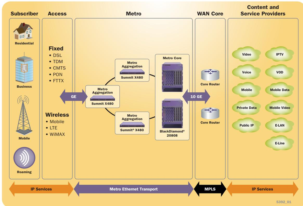
Figure 5: Summit X480 in a Carrier Ethernet Application
