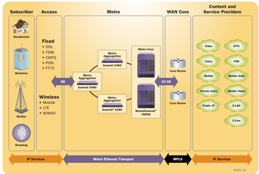
Figure 13: Summit X480 in a Carrier Ethernet Application
