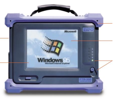
Shock-absorbing bumpers offer a high degree of protection in the field. The FTB-300 UTS meets all Bellcore drop-test requirements.
