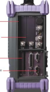
The UTS hosts up to three field-interchangeable test modules.
