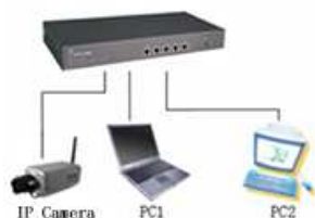
Picture 11 IP camera is connected to network via switch
