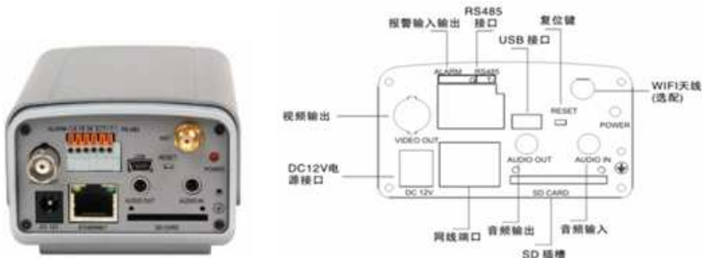
Picture 1 back view of box IP camera Picture 2: back panel illustration of box IP camera
