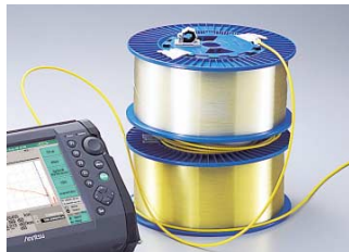
188 km optical fiber cable
